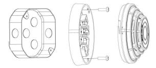
Smoke detector FW500/501 can be used with 12 AWG to 18 AWG.
